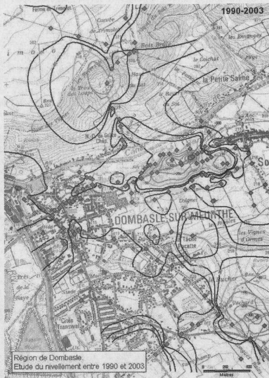
Figure 10. Sinking (in mm) in the Dombasle region (Nancy basin) between 1990 and 2003 (INERIS document)
